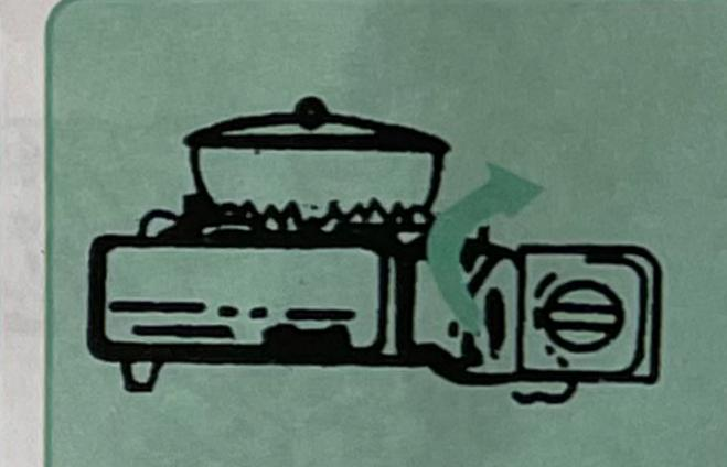
When you switch the button to the left the gasflame Will be turned on. To turn the gasflame off you switch the button to the right,
